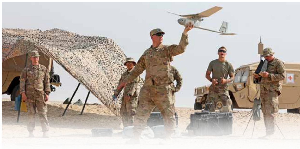
Army Soldiers prepare to launch the RQ-11 Raven. The Raven is a hand-launched, remote-controlled unmanned aerial vehicle that can be used for surveillance and reconnaissance, enabling units to gather information with reduced risk to Soldiers. U.S. Army photo by SGT Liane Hatch.
